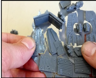
To start snap the waste resin off the parts.
