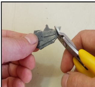
Clip the remains of the waste resin from the parts
