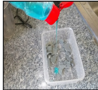
The resin may have release agent or dirt on it, so clean the parts with detergent.
