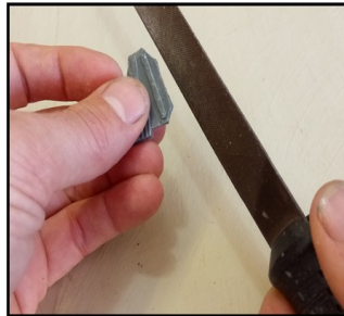
Use a metal work file to remove the sharp edges.
